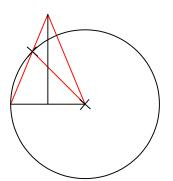
Draw a circles that uses the Octagon side wall length end point for the center of the circle and the length of the Octagon side wall length as the radius of the circle
