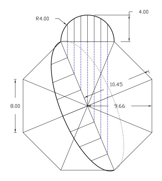
Octagon vaulting with Equal Side Lengths With Transverse ribs Semicircular Octopartite vaulting with equal height ordinates
