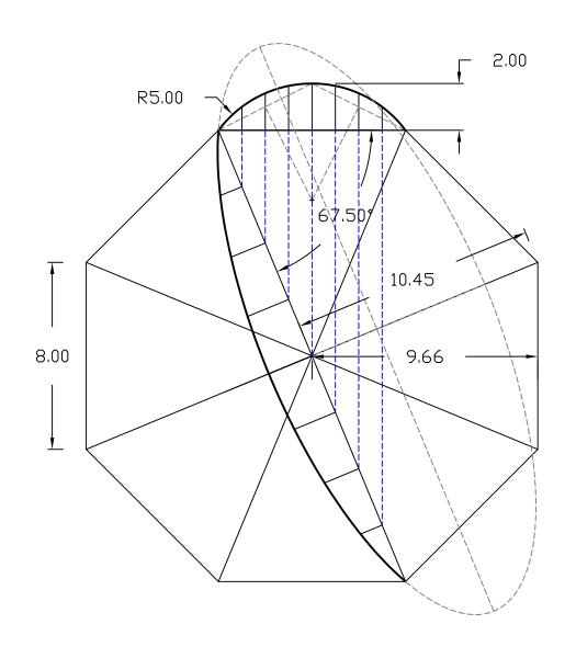
Octagon vaulting with Equal Side Lengths With Transverse ribs Segmental Octopartite vaulting with equal height ordinates
