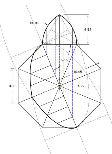
Octagon vaulting with Equal Side Lengths With Transverse ribs Gothic Octopartite vaulting with equal height ordinates
