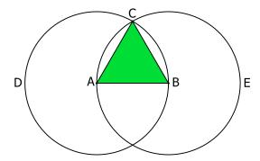
Euclid's Elements Book 1 Prop 1 To construct an equilateral triangle on a given finite straight line A-B.
