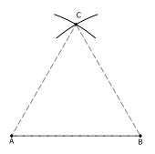
Draw Equilateral Arc AC from point B and Equilateral Arc BC from point A
