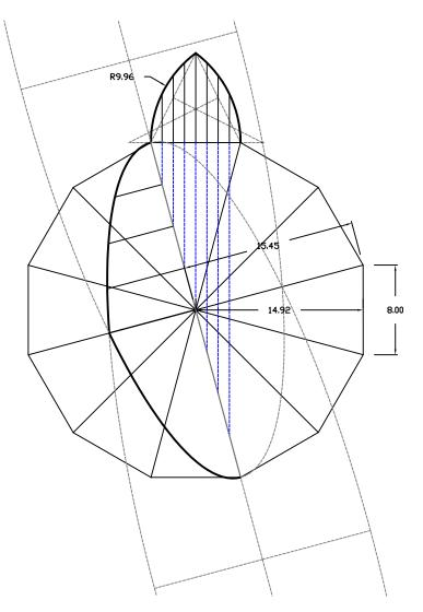
Dodecagon vaulting with Equal Side Lengths With Transverse ribs Lancet Gothic with equal height ordinates
