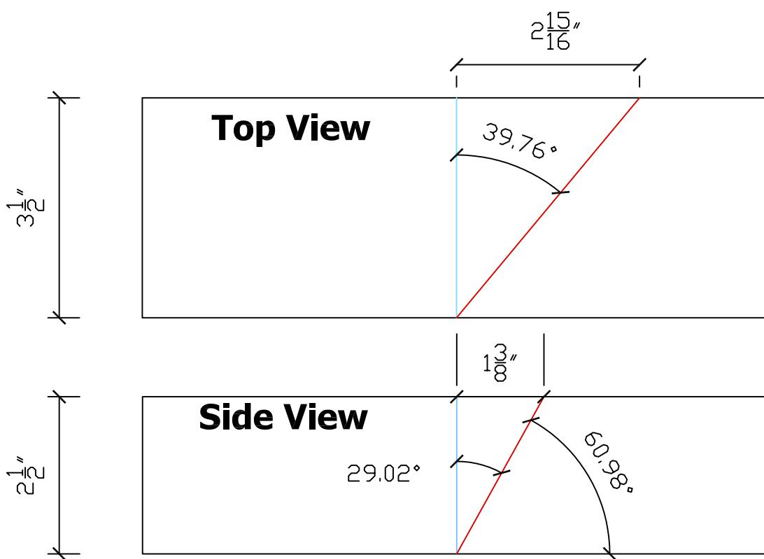
**Saw Blade Bevel of  $23.09^\circ$  produces
